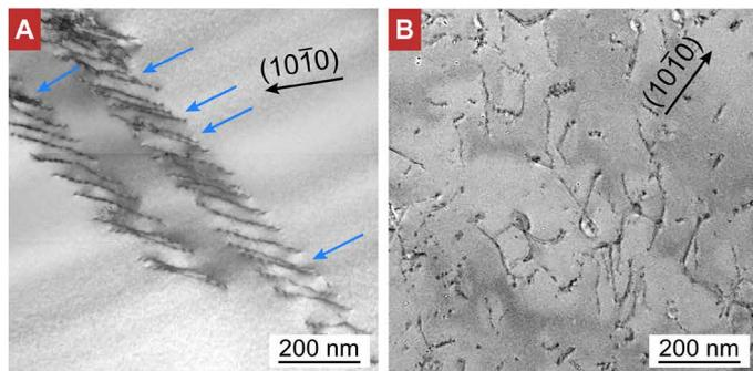
**Fig. 1. TEM bright-field imaging of deformed Ti-6Al with different thermal history.** (A) Sample aged to promote SRO; the blue arrows mark the in-band dislocation pairs. (B) Sample quenched after homogenization.
