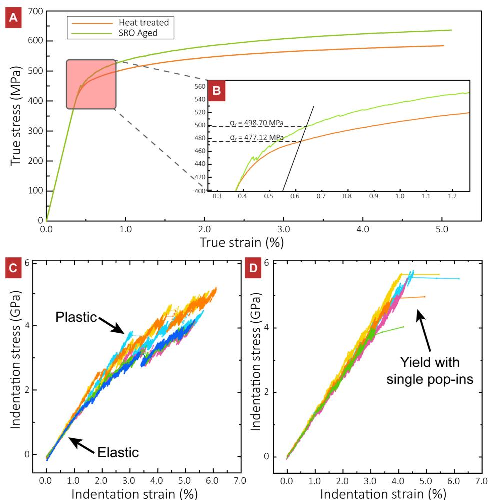
**Fig. 3. Comparison of the mechanical response of Ti-6Al in the quenched and SRO-aged conditions.** (A) True stress-strain curves of the quenched and SRO-aged samples. (B) Enlarged true stress-strain curves near yielding of both materials; the 0.2% offset yield strength is marked on the plot. (C and D) Indentation stress-strain curves of as-quenched sample and SRO-aged sample, respectively. Different indentations are marked with different colors.
