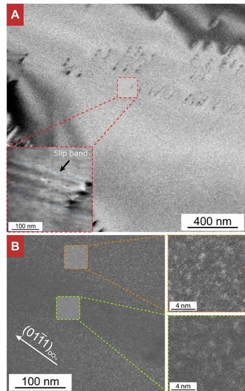
**Fig. 4. Energy-filtered DF images of planar dislocation slip bands.** (A) Bright-field image showing the relation of a slip band and the imaging area. The slip band is marked and shows weak-fringing contrast in the zoomed-in image. (B) Energy-filtered DF image at the same position of (A) showing the lack of contrast in the slip band.
